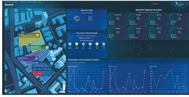
The Environmental Monitoring Module of the DCMP collects real time environmental data including noise and pollutant levels from different construction sites for URA staff's monitoring from their offices.
